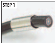
STEP 1 Cut cable to length and slide crimp ring onto free end.
