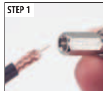
STEP 1 Prepare cable with strip tool.
