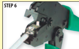
Crimp plug with the specially designed HTS2500 or HTS2600 crimp tool.
