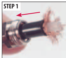
STEP 1 Cut cable and slide nut into position. Strip and flair braid.
